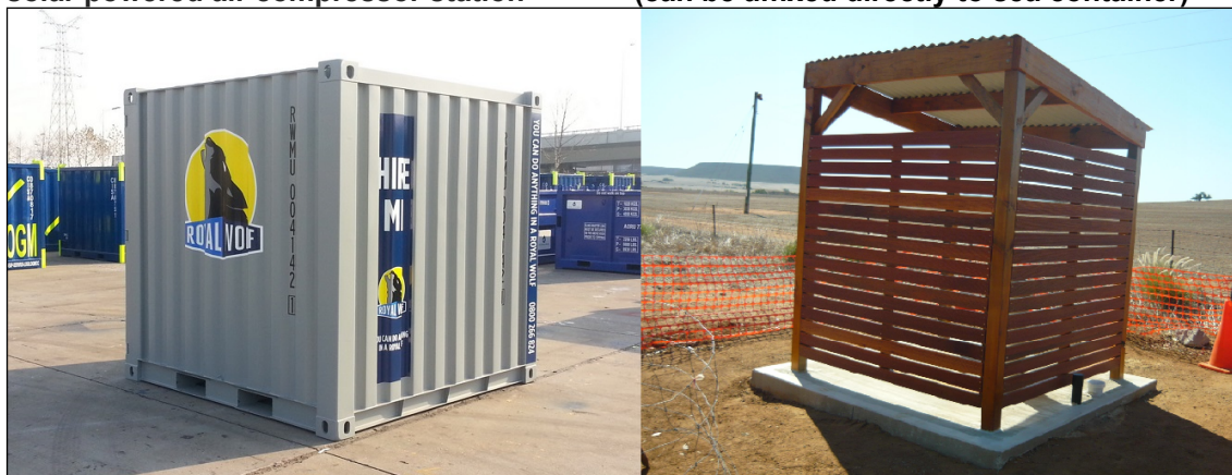
Figure 10.1.3(b) Proposed sea container to house solar powered air compressor station potential style of cladding for sea container (can be affixed directly to sea container)
