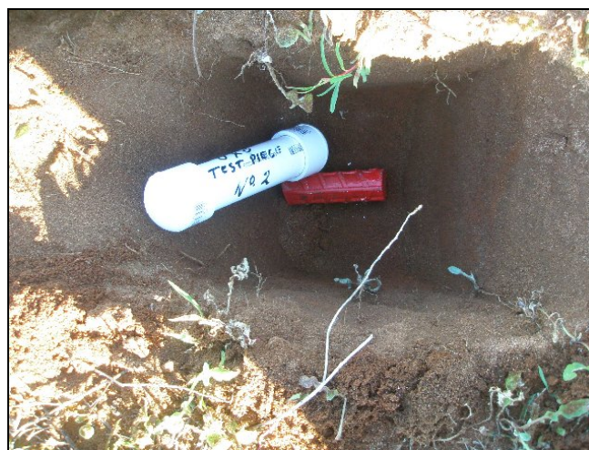
Photograph 5: 20mm Cannon Projectile Representative Test Piece buried at 200mm
