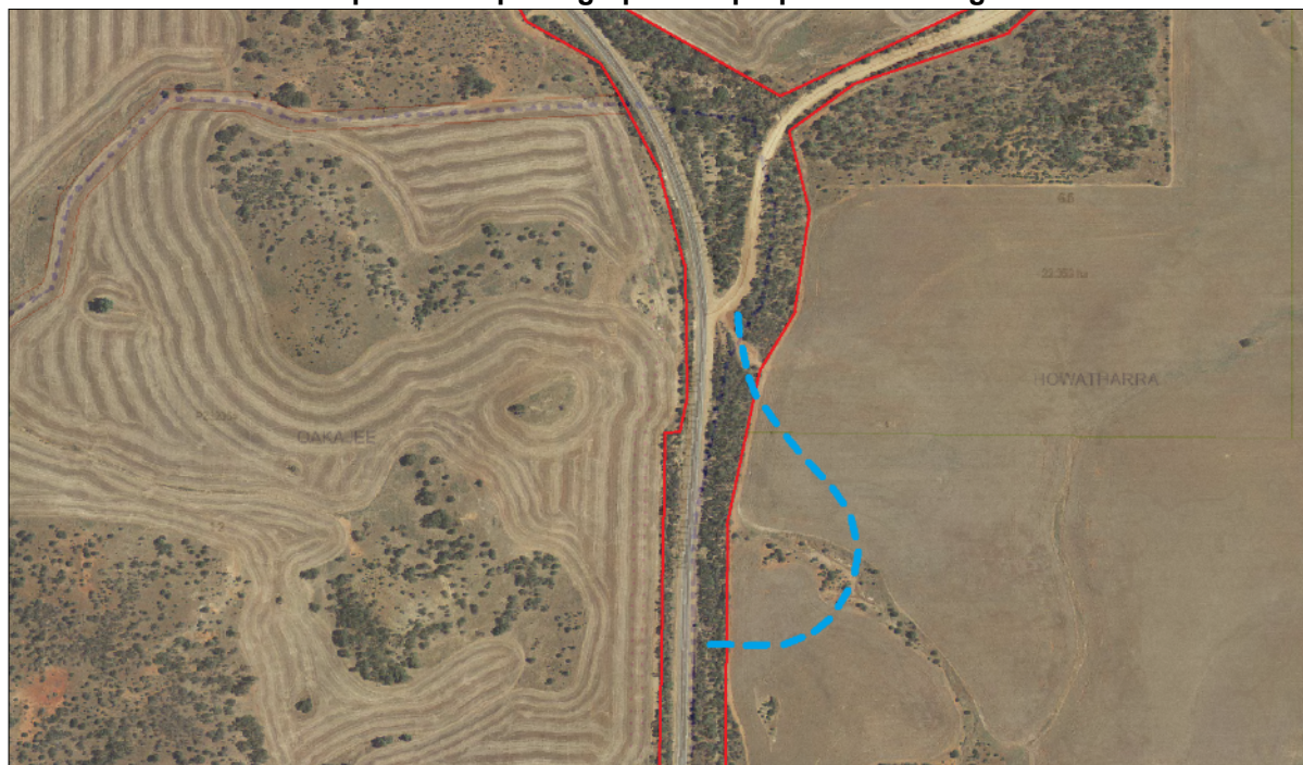
Figure 9.1.5(a) – Existing cadastral boundaries for North West Coastal Highway and Olsen Road reserves overlaid upon aerial photograph with proposed new alignment indicated in blue
